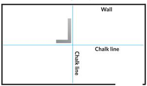
2. Find the arrowhead-shaped corner on each Pro-Fit tile. *Tiles must be installed with the arrowhead corners all "pointing" in the same direction.*
